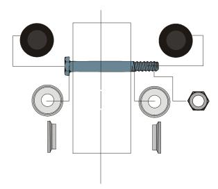
Figure 10. Pulley bolt assembly configuration.
